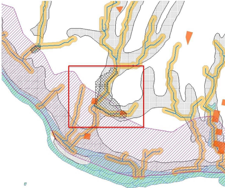
Figure 3a.4. Areas of overlap between the various wetland indicator layers. Each wetland indicator layer was assigned a score. Areas with the greatest number of overlapping indicator layers received higher overall scores and are therefore more likely to be wetlands (Figure 3a.4). This process was piloted in the Bennett Creek watershed, which is located in the southern portion of Frederick County (Figure 3a.5).
