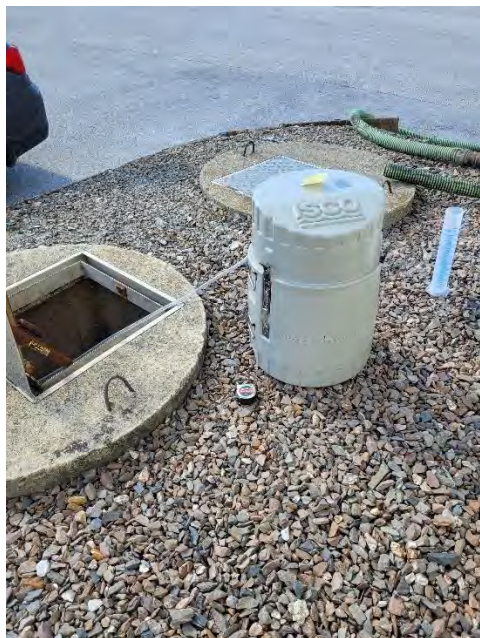
Figure 12. Stone autosampler setup for collecting a manually flow proportioned sample.
