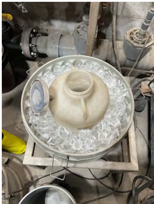
Figure 8. St Albans Creamery, LLC sample collection jug in base of autosampler.
