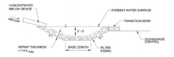
Figure 6-9. Plunge Pool, Rectangular (Profile View), Design Guidance (Source: NCDOT 2014)
