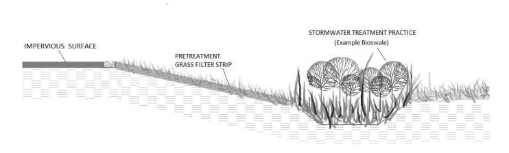
Figure 4-2. Pre-Treatment Filter Strip, Design Guidance
