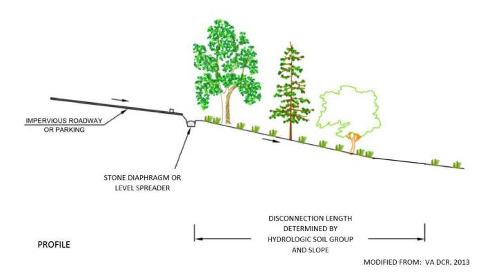
Figure 4-6. Disconnection to Filter Strips and Vegetated Buffers, Design Guidance
