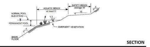
Figure 4-18. Shallow Surface Wetland, Design Guidance
