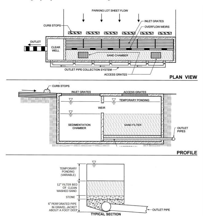
Figure 4-17. Perimeter Sand Filter, Design Guidance
