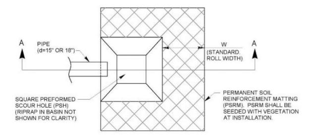
Figure 6-6. Plunge Pool (Plan), Design Guidance (Source: NCDOT 2014)
