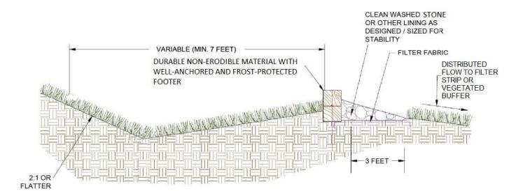
Figure 4-8. Disconnection to Filter Strips and Vegetated Buffers, via Level Spreader, Design Guidance
