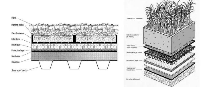
Figure 4-23. Extensive Green Roof (L) & Intensive Green Roof (R), Design Guidance (Source: Wark and Wark 2003)
