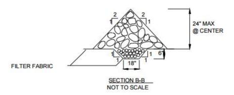
Figure 6-11. Check Dam (Detail), Design Guidance
