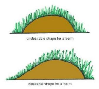
Figure 6-2. Infiltration Berm Shape, Design Guidance
