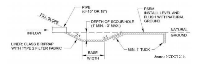
Figure 6-7. Plunge Pool (Profile), Design Guidance (Source: NC DOT 2014)
