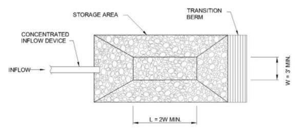
Figure 6-8. Plunge Pool, Rectangular (Plan View) Design Guidance (Source: NCDOT 2014)
