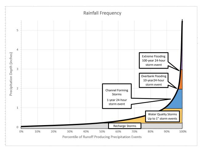
Figure 2-1. Approximate Ranges for Storms Comprising Treatment Standards Sizing Criteria, Design Guidance
