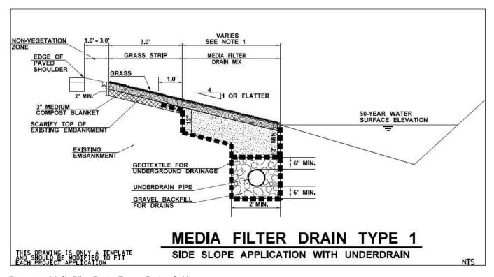
Figure 6-3. Media Filter Drain, Type 1, Design Guidance
