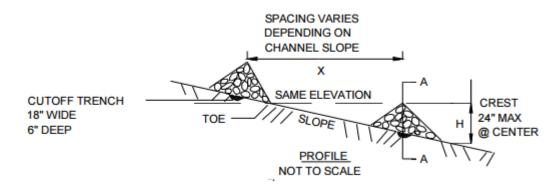
Figure 6-10. Check Dam (Profile), Design Guidance
