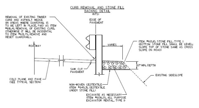
Figure 6-1. Curb Removal (Detail), Design Guidance
