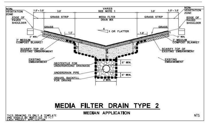
Figure 6-4. Media Filter Drain, Type 2, Design Guidance
