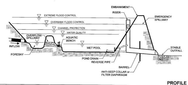
Figure 4-20. Wet Pond, Design Guidance
