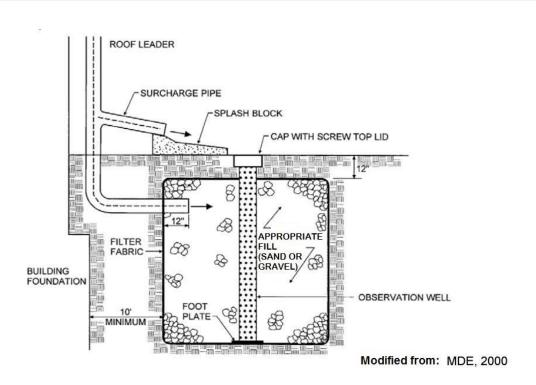
Figure 4-12. Dry Well, Design Guidance
