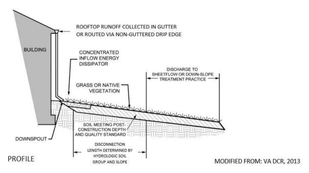
Figure 4-5. Simple Disconnection, Design Guidance
