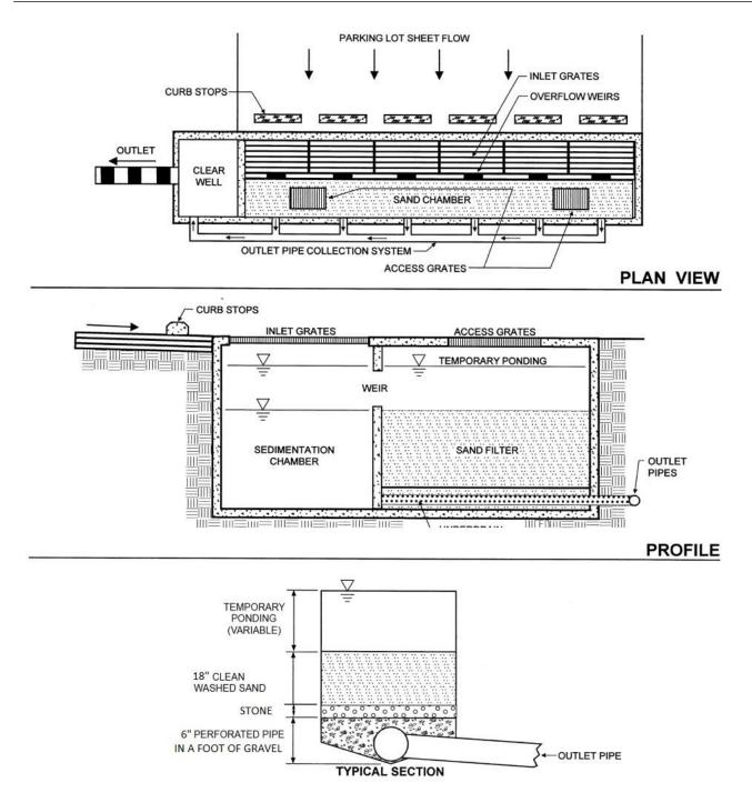
Figure 4-16. Underground Sand Filter, Design Guidance
