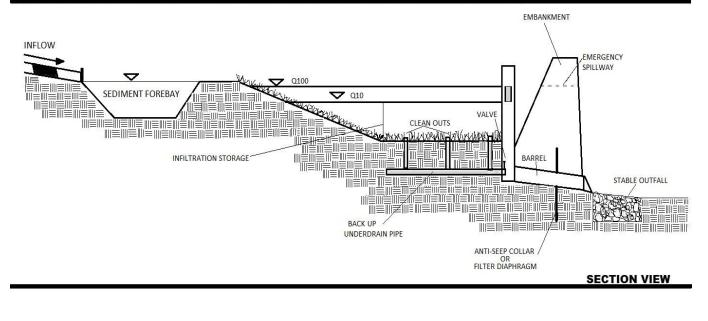
Figure 4-13. Infiltration Basin, Design Guidance
