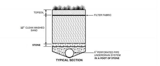
Figure 4-15. Surface Sand Filter, Design Guidance
