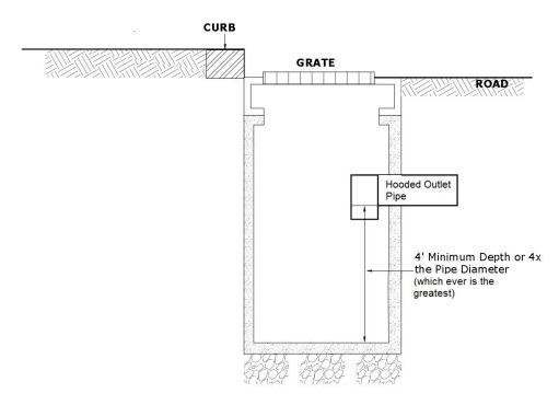
Figure 4-4. Deep Sump Catch Basin, Design Guidance
