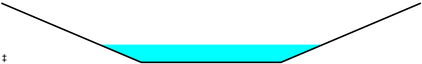
Reach 9R: Treatment Swale
