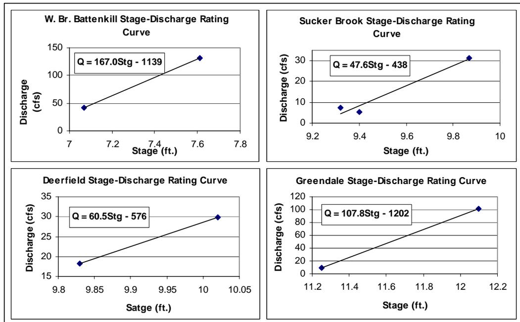
Figure 1. Stage-discharge rating curves for study sites.
