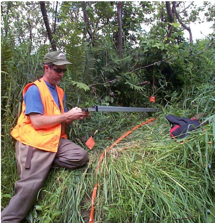
Figure 4 Lateral bar indicating bankfull stage. Note that the upslope flag is location of bankfull stage. At this location the slope of the bar surface becomes nearly flat. Also note the woody vegetation line at that point.
