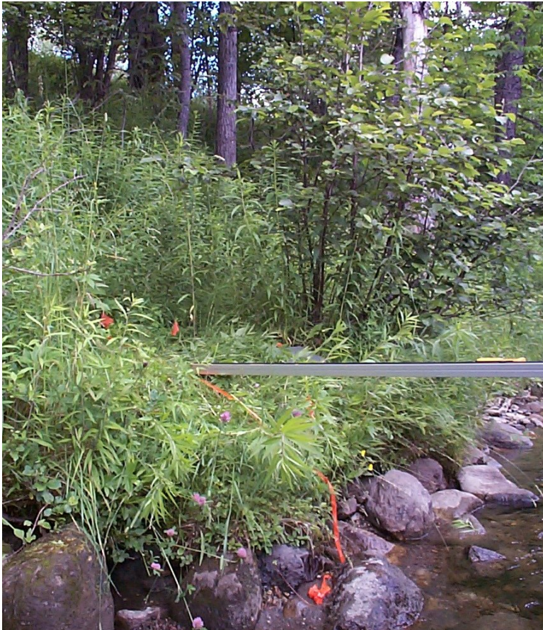
Figure 6 Bench feature indicating bankfull. Survey rod shows the slope of the bench surface.
