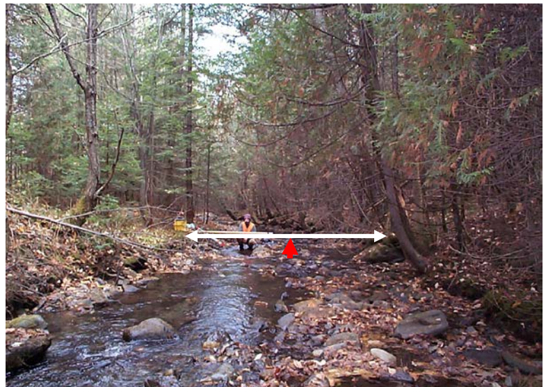
Figure 1. Bankfull elevation on a steep upland stream at which bankfull channel width measurements are taken.
