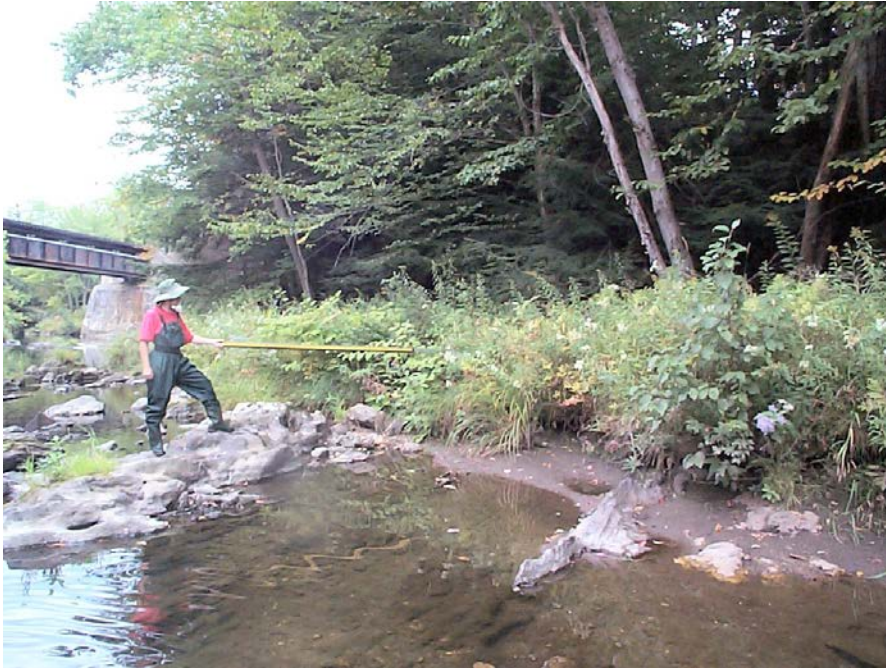
Figure 3 Close up of Figure 2. Survey rod shows slope (nearly flat) of the lateral bar surface.
