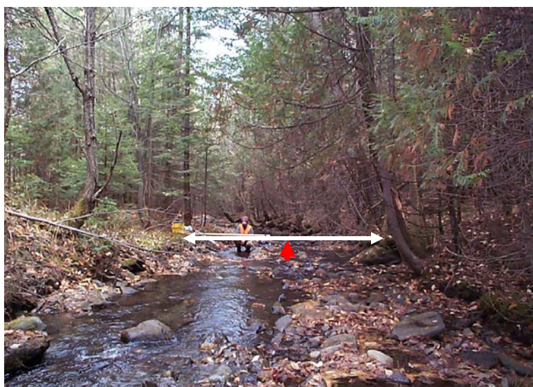
Figure 1. Bankfull elevation on a steep upland stream at which bankfull channel width measurements are taken.
