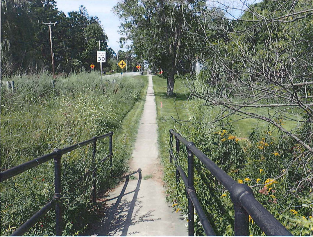
Photo 3. View westward from the Allen Brook pedestrian bridge. Williston Road is on the left. The proposed force main would be directional bored under Allen Brook and its riparian wetlands. Open trenching for force main installation would begin in the lawn and run to the sewer manhole beyond the tree to the right of the sidewalk. (August 24, 2016)
