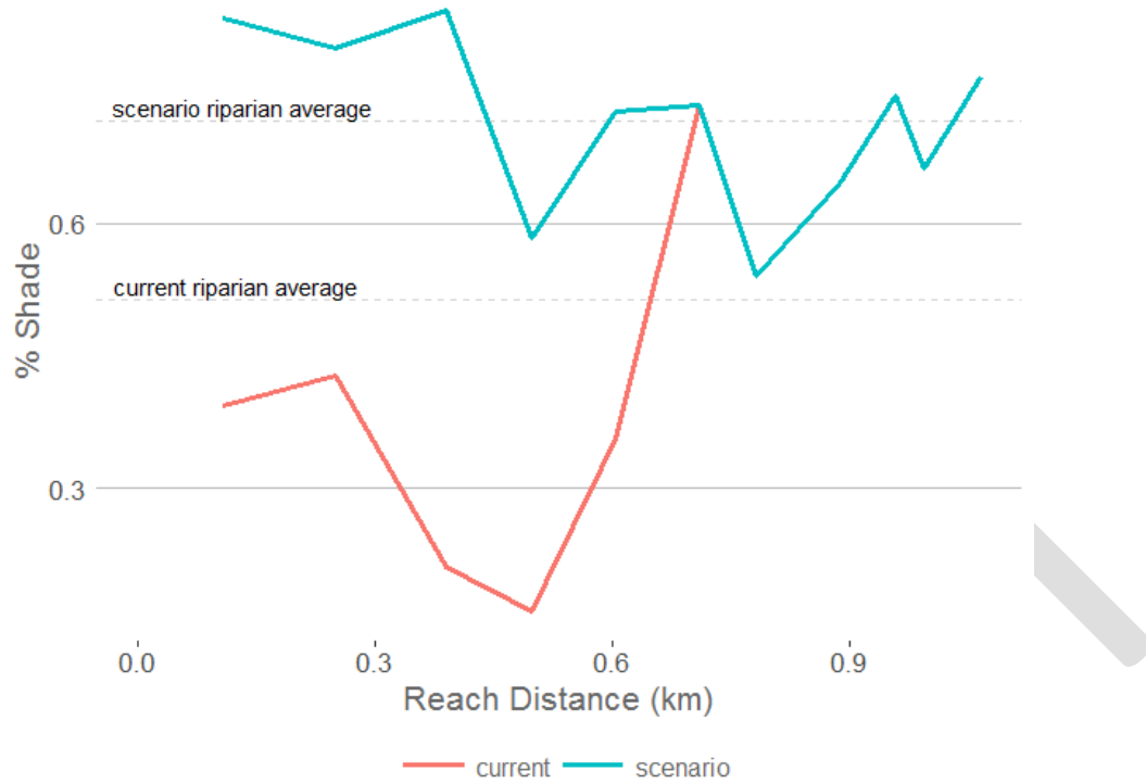
Figure 15 Comparison of average percent shade by reach for current conditions and TMDL scenario. Dotted lines represent average percent shade over the modeled reach.
