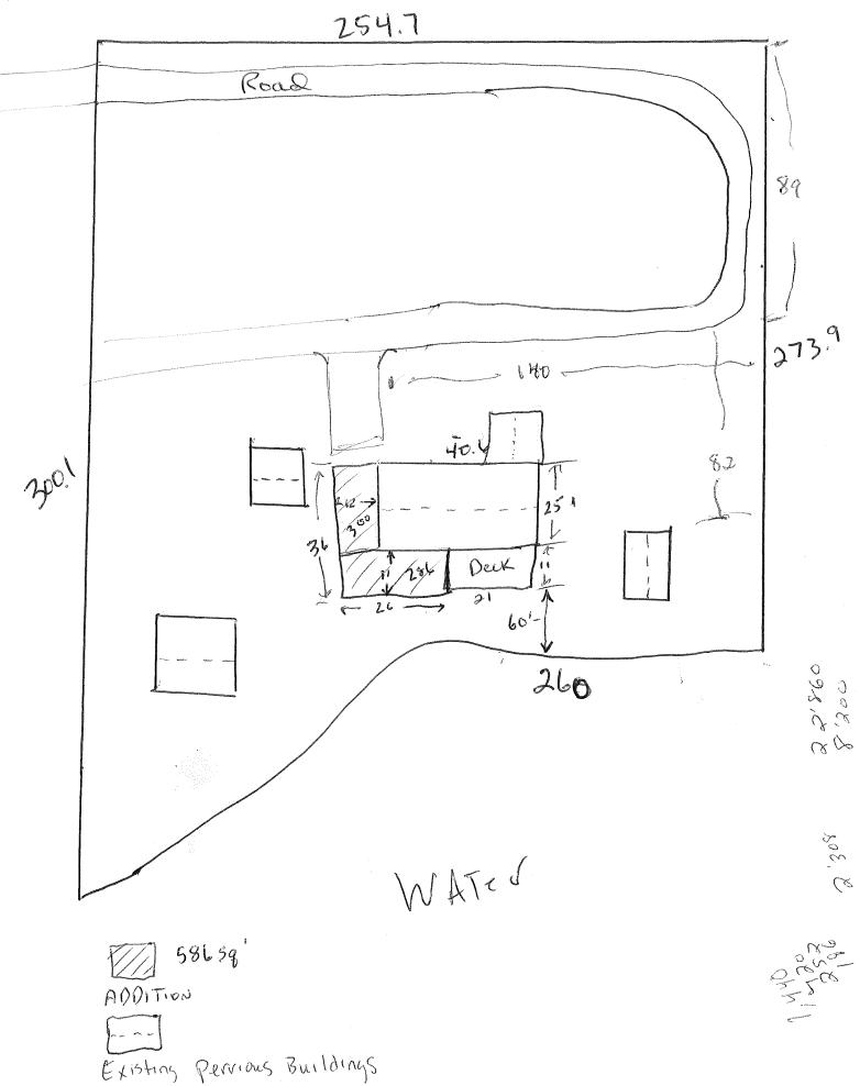
PLOT TO SCALE: THE EXISTING BUILDINGS AND THE PROPOSED CONSTRUCTION, FRONT (TO THE CENTERLINEOF THE ROAD), BOTH SIDE YARD SETBACKS, REAR YARD SETBACK, AND ALSO A COMPASS ARROW SHOWING N,E,S,W.
