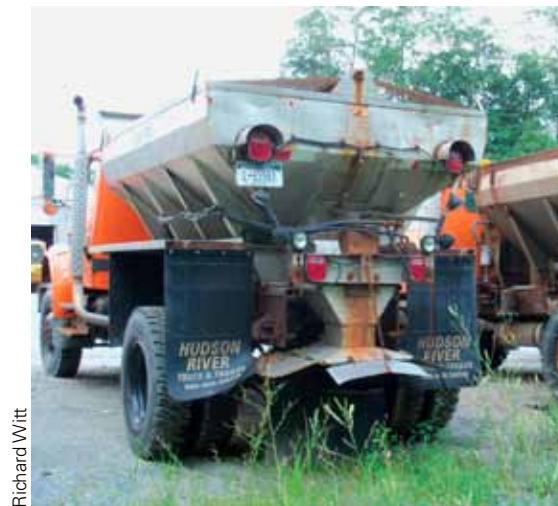
There are several manufacturers of road deicing equipment. The control units are installed in the cab of the truck, which regulate the dispersal of the sand or chemical in the spreader.
