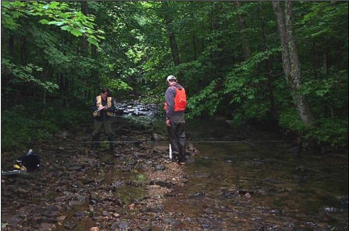
Figure 21: Typical cross-section along reach T6.07. Note the abundant fine sediment that has filled in much of the stream bottom. Habitat in this reach was rated as fair due to excessive sediment and lack of deep pools.
