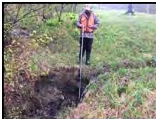
3-ft deep headcut has developed (05/22/2014)
