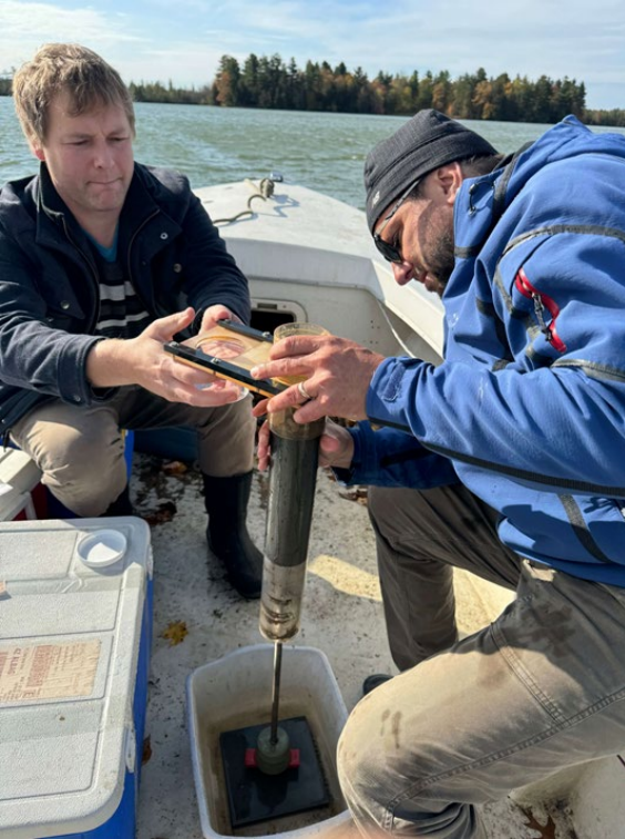
Figure 3-2 Photograph demonstrating the sediment coring tube, stand, and slicing device used in this study
