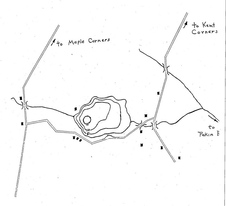
Depth Survey performed using depth tape along 3 transects; 1 east-west, and 2 north-south. By Eric Swanson, Vermont Department of Water Resources and Environmental Engineering, Montpelier. May 31, 1982.
