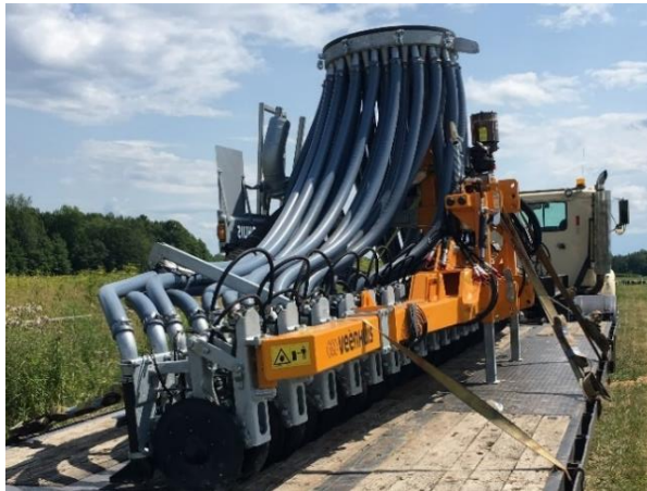
Figure 6. Grassland shallow slot manure injector to be used within the Lake Carmi watershed. Manure is injected subsurface to reduce surface runoff of nutrients. Equipment funds were awarded in SFY 2020 and will be reported in future Lake Carmi Clean Water Progress Report updates.
