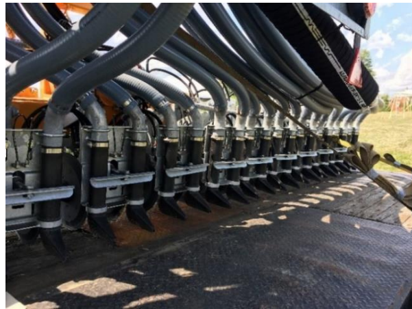
Figure 6. Grassland shallow slot manure injector to be used within the Lake Carmi watershed. Manure is injected subsurface to reduce surface runoff of nutrients. Equipment funds were awarded in SFY 2020 and will be reported in future Lake Carmi Clean Water Progress Report updates.
