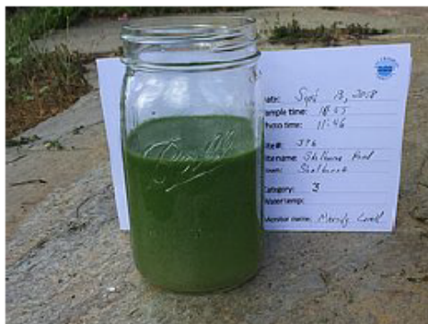
3. Close-up of jar water sample after performing 30-minute jar test.
