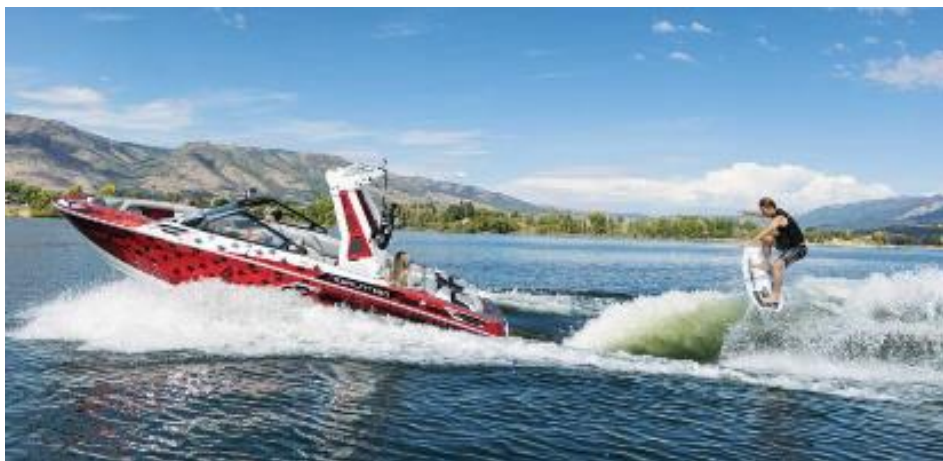
Figure 5: Bow-up orientation of the wake boat creates line-of-sight vision issues
