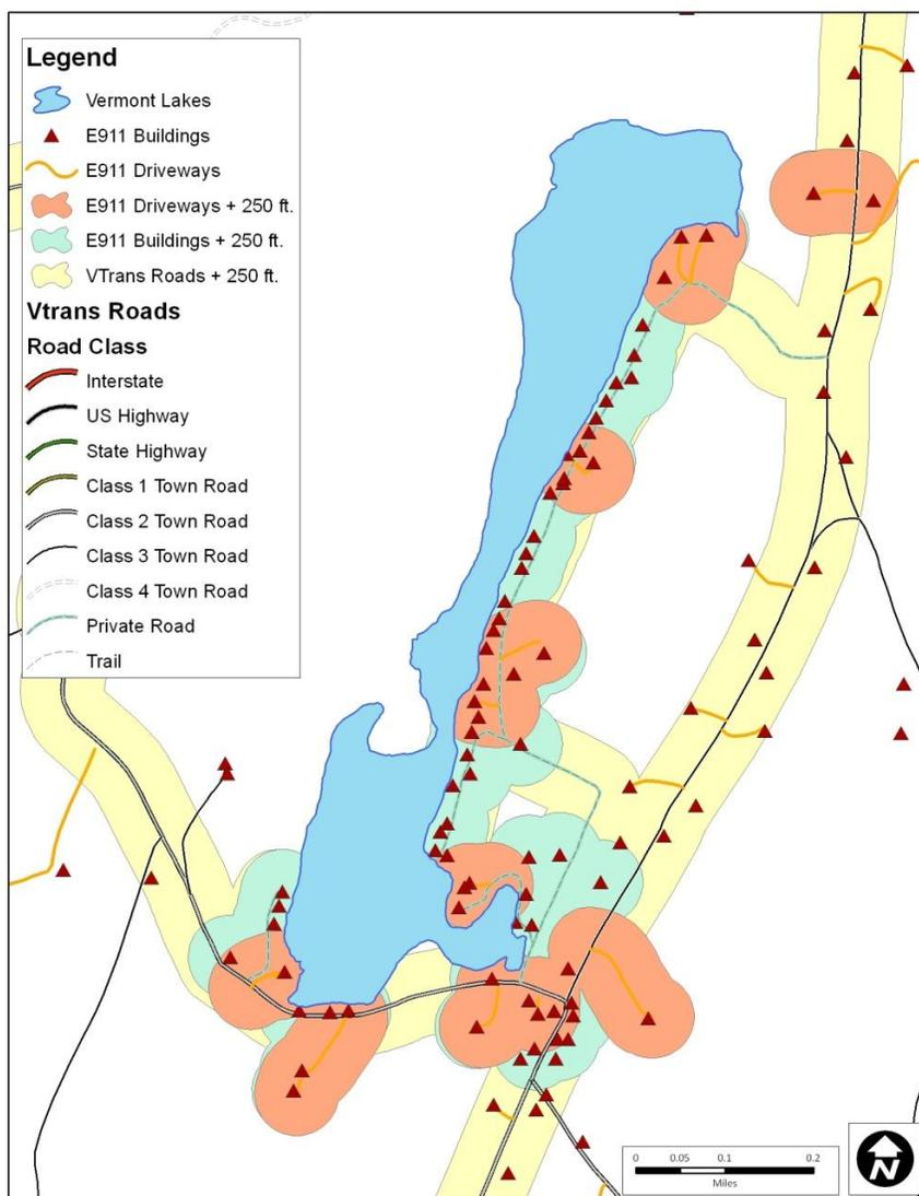
Figure 1. An additional 250 ft. was added to locations of buildings, driveways and roads located near lakes to determine the areas of impact near lakeshores.
