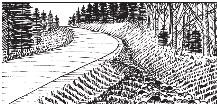
Ditched turnouts channel water away from the road into vegetated buffers.
