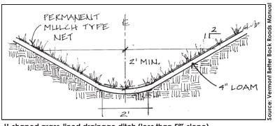
U-shaped grass-lined drainage ditch (less than 5% slope).
