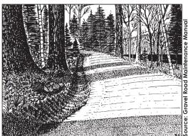
Crowned driveway with a rock-lined drainage ditch.
