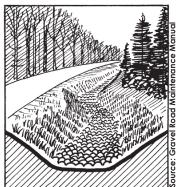
Use grass and stone to control erosion for ditches with more than 5% pitch.
