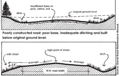
Crown profile:  $\frac{1}{2}$  of crown per foot of road width from the center. (e.g. 10 ft/2 = 5 ft high point of crown, 5 ft x 1/2" = 2 1/2" crown height).
