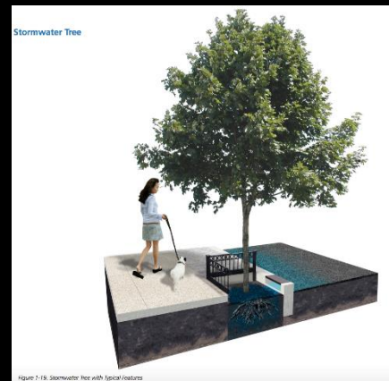
Storm Water Tree Pits
