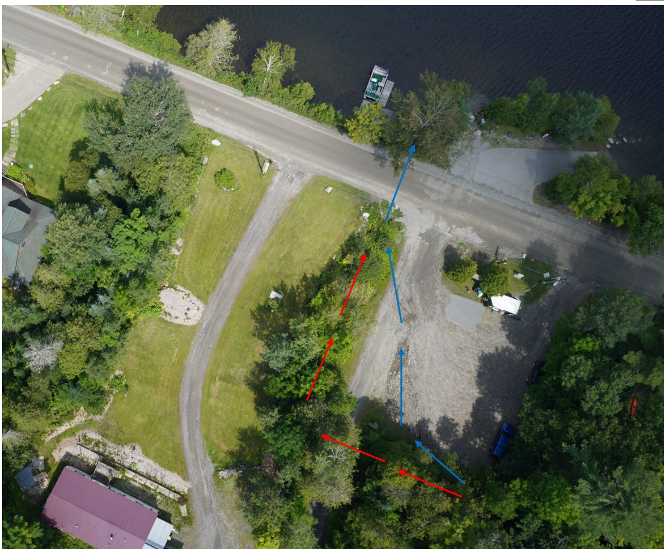
Figure 31. The tributary along the Fish and Wildlife Access area (shown with red arrows) jumped its banks and flowed through the parking area during the July 2023 storm (blue arrows).
