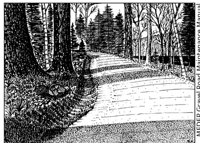
A crowned driveway encourages sheetflow of runoff to stable upslope drainage ditches and downslope buffers, minimizing erosion of road surface.
