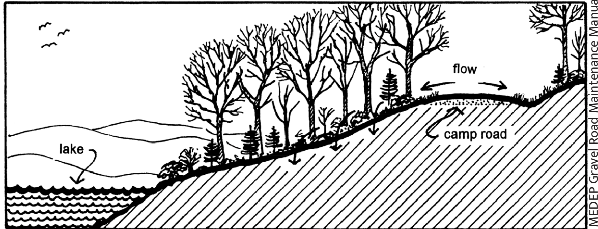
Road runoff is dispersed and absorbed by nearby stable vegetated buffers.
