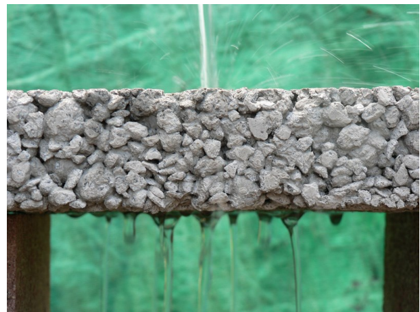
WATER PASSING THROUGH PERVIOUS CONCRETE, ANOTHER FORM OF POROUS PAVEMENT
