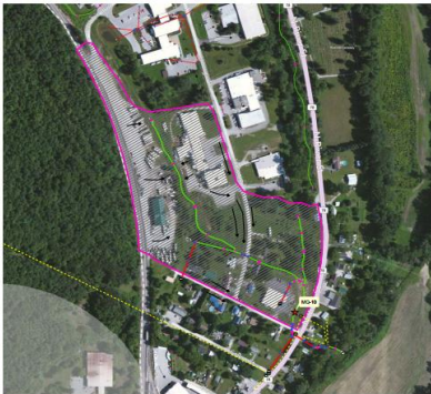
Figure 4. Subwatershed drawing to a culvert at the southeast corner of the Fountains Door and Window business at the corner of Rt. 78 and Brooklyn St.
