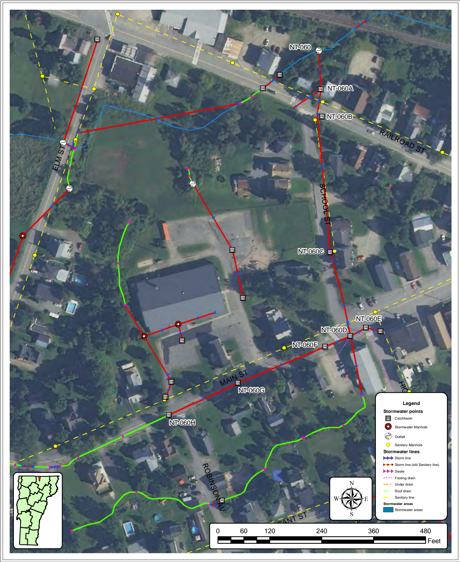
Figure 5. Stormwater drainage system discharging at outfall NT-060 North Troy, VT
