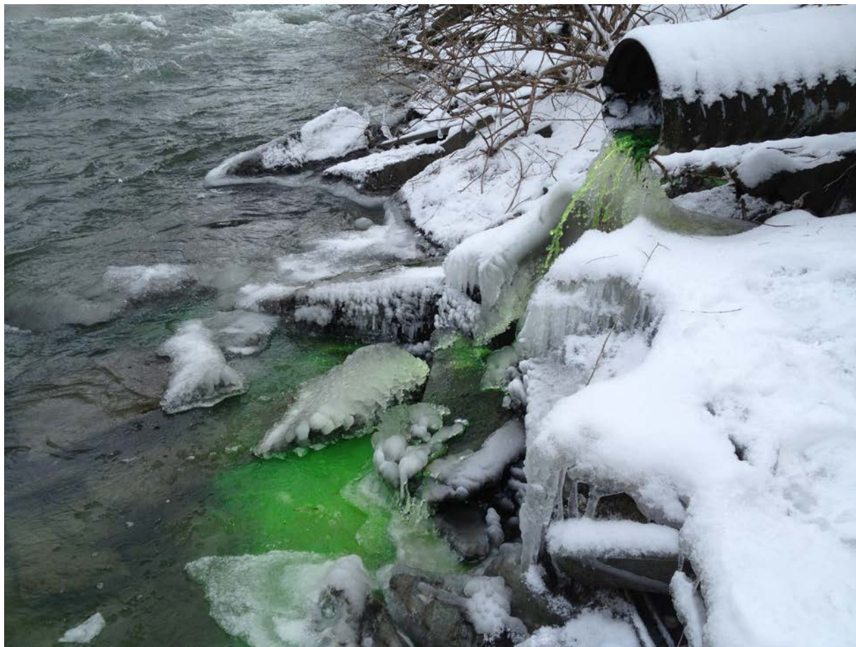
Dye flushed down a toilet in Fair Haven discharges to the Castleton River at outfall FH280, confirming presence of a sanitary wastewater connection
