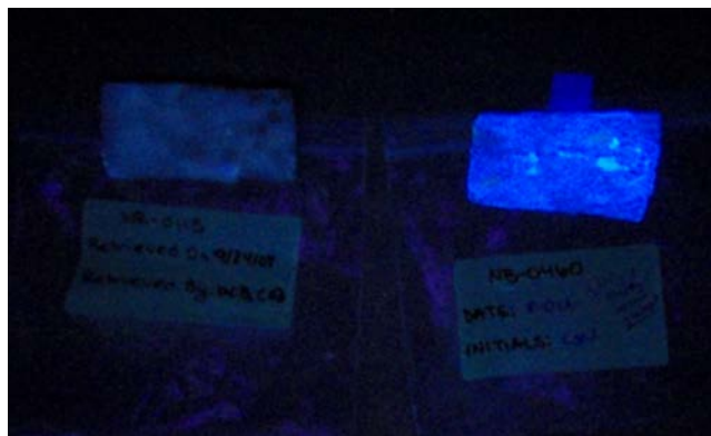
Figure 1. Optical brightener monitoring pads under UV light
