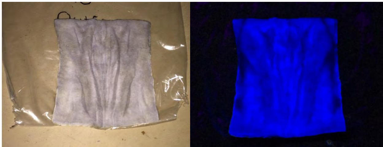
Figure 1. Positive optical brightener pad under fluorescent (left) and UV (right) lamps.
