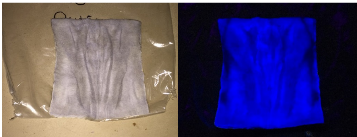
Figure 1. Positive OB pad under fluorescent (left) and UV (right) lamps
