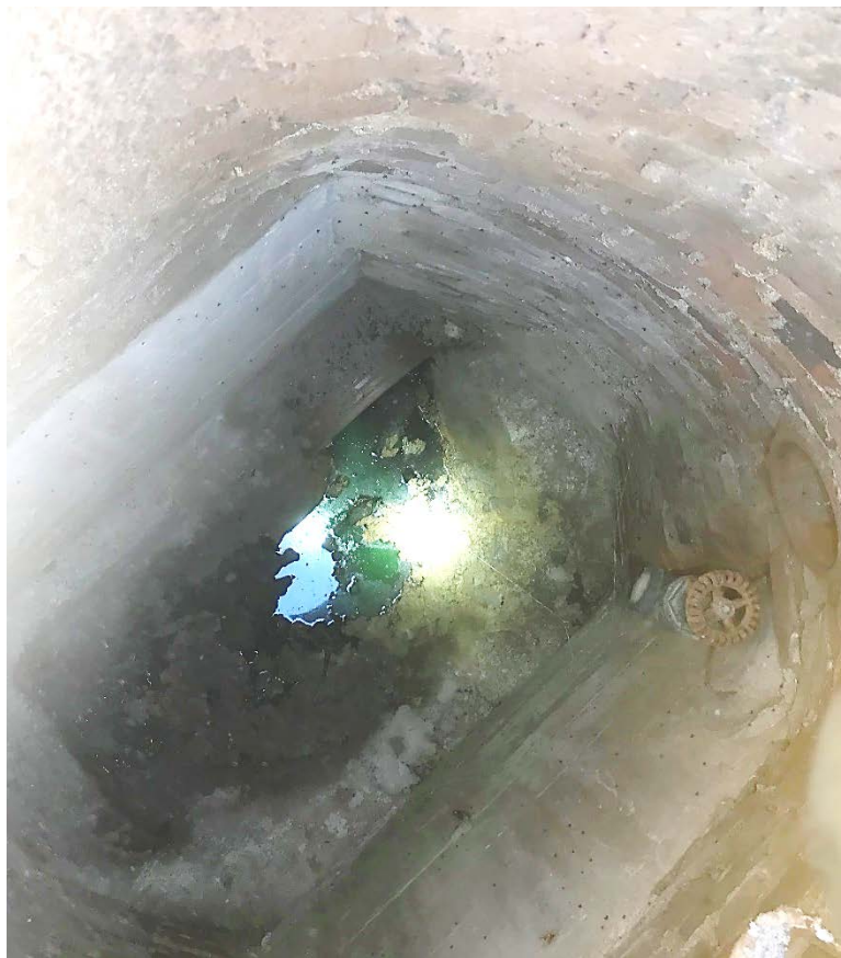
Figure 2. Dye in stormwater MH-4 after flushing in Wooley dorm
