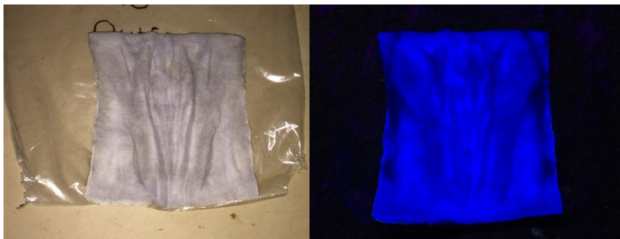
Figure 1. Positive optical brightener monitoring pad under fluorescent (left) and UV (right) lamps.
