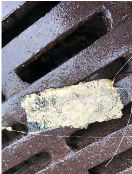
Figure 5. Optical brightener pad coated in sawdust from CB10 sump
