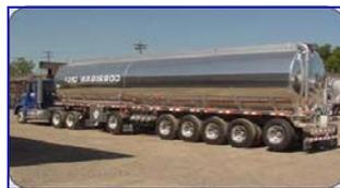
Larger volume deliveries are done with tanker trailers or tanker trucks which fill tanks with a passive gravity feed system. When receiving del-
