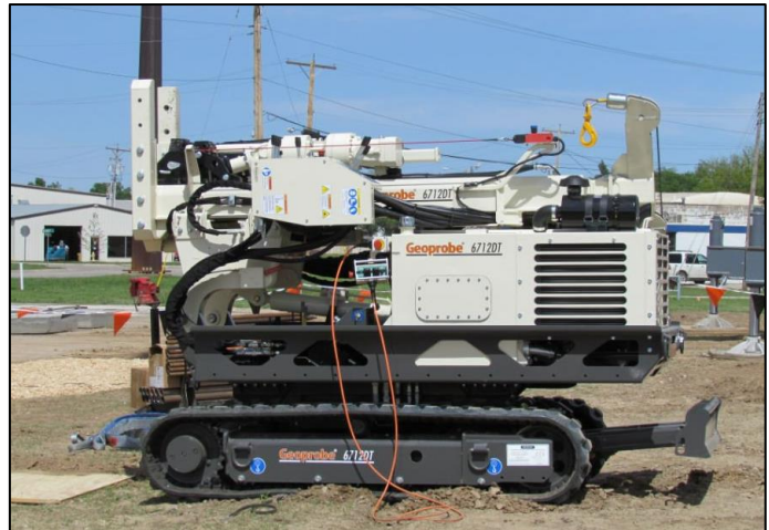
An example of a Direct Push Technology drilling rig used for collecting subsurface soil samples. www.geoprobe.com
