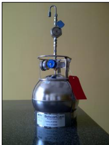
A typical canister used to collect indoor air or soil vapor samples. www.itrcweb.org
