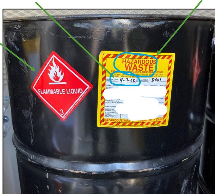
On the drum above, note the clear indication of the hazard ("flammable"), date, and words "Hazardous Waste." This would be appropriate for storage in an STSA.
