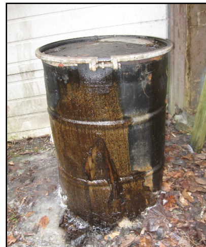
Above: freezing and expansion of the drum's contents has caused it to rupture (center), resulting in a release to the environment.
