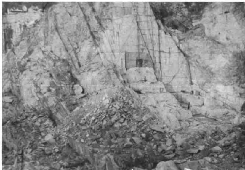
Plate 23. Major joints in the Barre granite—strike N50-70^{\circ}E , dip 55-80^{\circ}SE . View on a south-facing wall of the Rock of Ages quarry.
