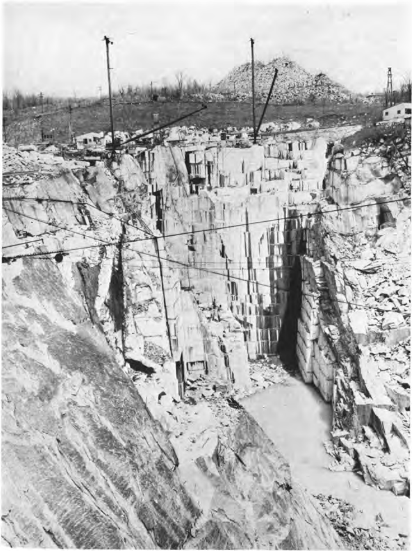
Rock of Ages Quarry seen from its southwestern end. Prominent joint surfaces and a dark dike cutting the Barre granite are seen in the left side of the photograph. Grout piles in the background.
