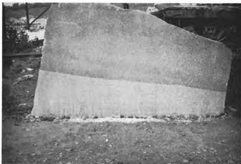
Plate 16. Sharp contact between 'dark' and 'light' granite. Faint banding observable in the dark granite. Exhibition (polished) slab Rock of Ages quarry.
