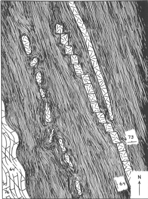
Figure 2. At Cobb Brook on west side of Pine Hill road. Three stages in disruption of granite streamers in slates of the Barton River formation. Disruption of one streamer has advanced to the boudinage stage. The sketch covers a width of 8 feet.
