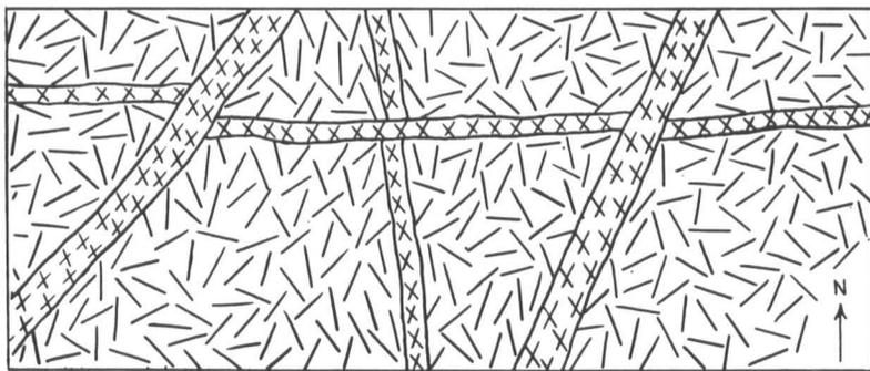
Figure 3. Southeast slope of Barton Mountain on north side of Barton-Lake Willoughby highway,  $1\frac{1}{4}$  miles west of elevation 1404. Three generations of pegmatite veins in granite. The sketch covers a width of  $5\frac{1}{2}$  feet.
