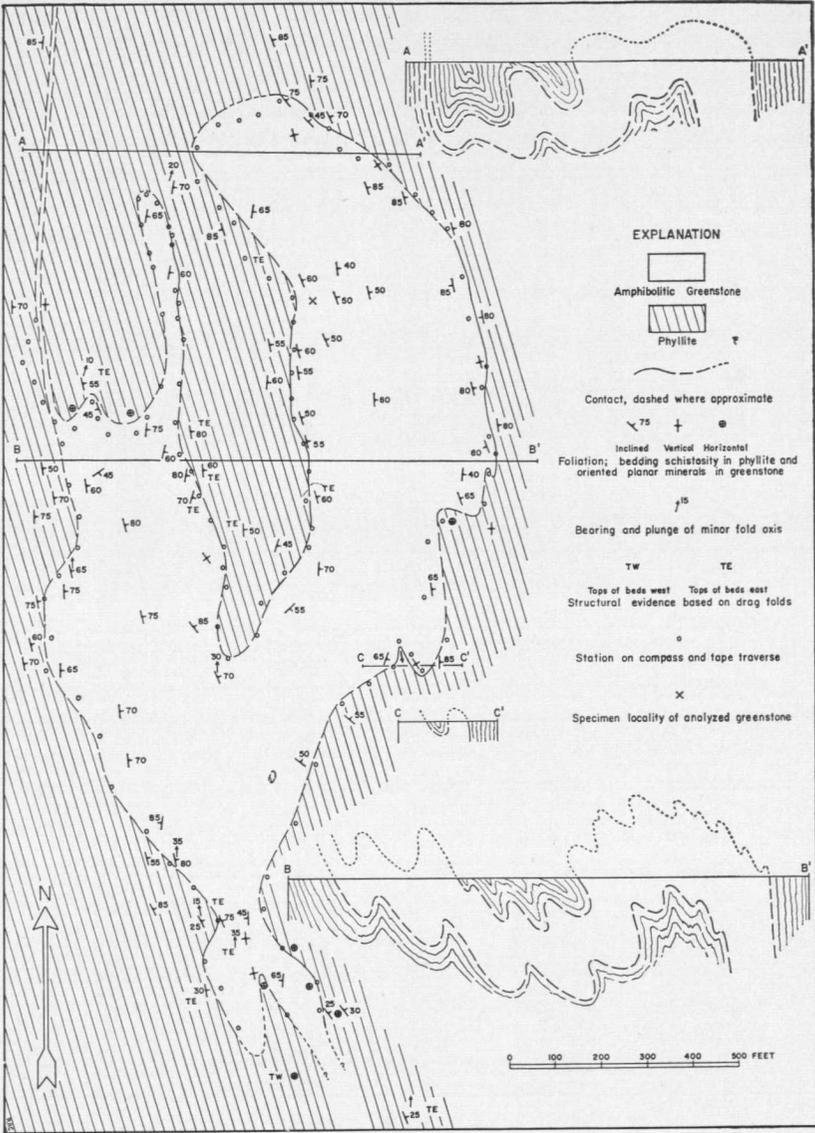
Figure 3. Geologic Map of the Amphibolitic Greenstone, South of Gillett Pond (Loc. 24, Fig. 2).
