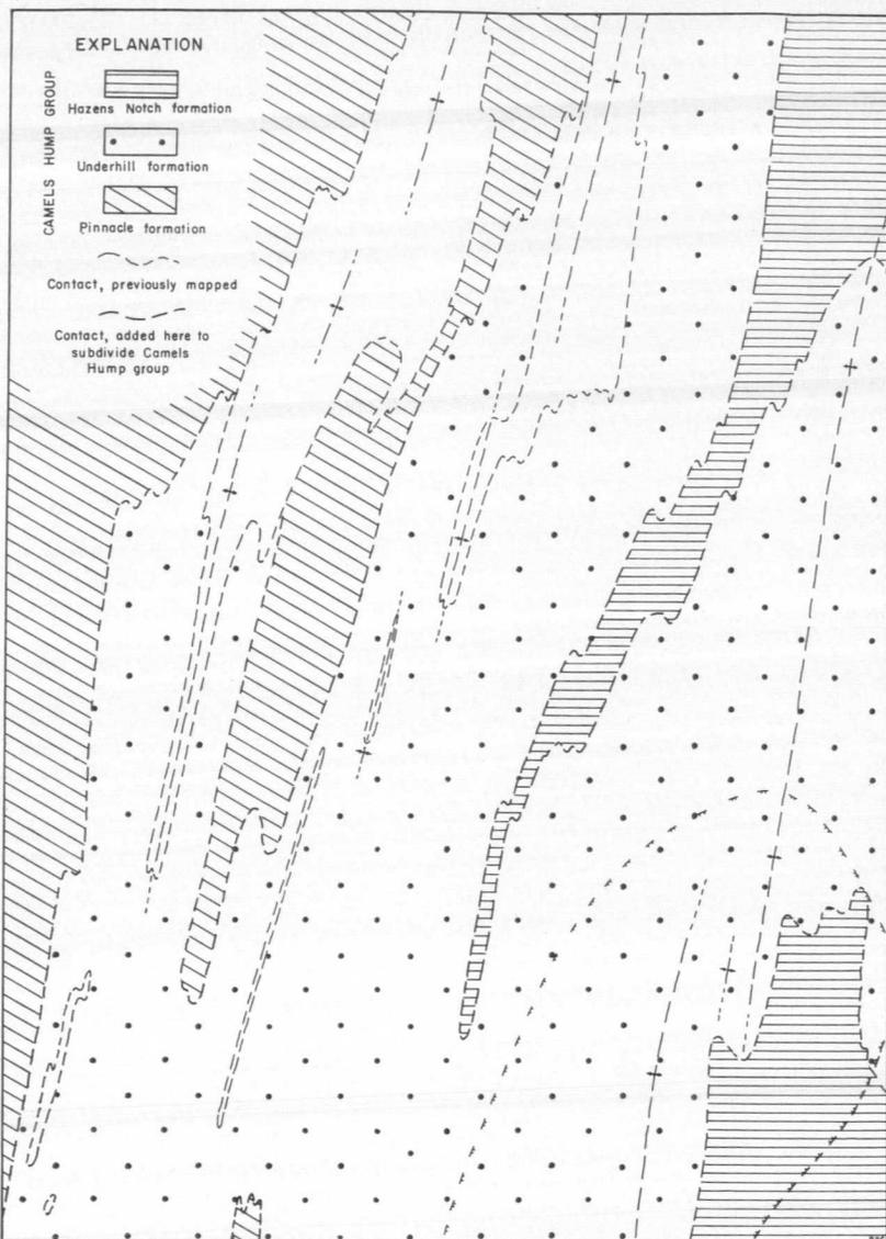
Figure 4. Geologic map of the Mount Mansfield Quadrangle showing the subdivision of the Camels Hump group into the Pinnacle, Underhill and Hazens Notch formations.
