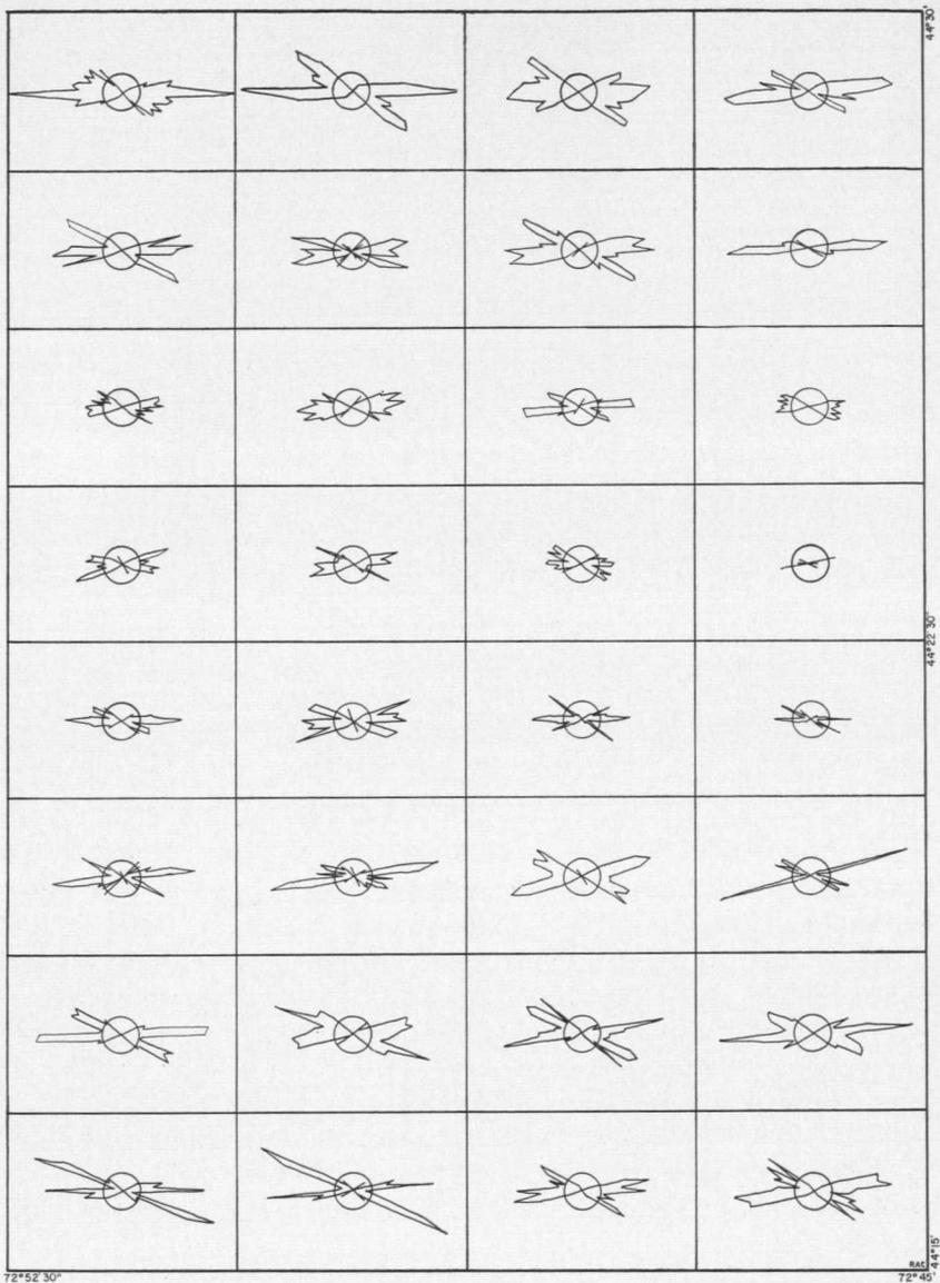
Figure 7. Joints from aerial photographs, east one-half of the Camels Hump quadrangle. Each circle has a radius which represents five joint lineations, and each of the 32 patterns records the joints measured in equal area in the eastern half of the 15' quadrangle. The relative position of the areas is shown but the size and shape of the areas are distorted in this illustration.
