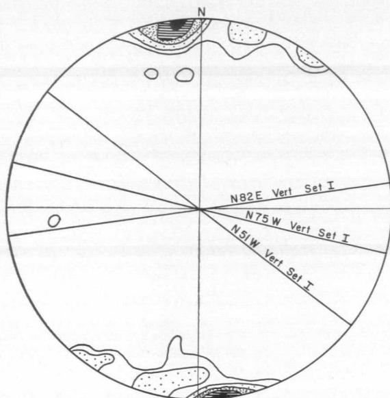
Figure 6. Joint diagram, Huntington Falls (Loc. 38, Fig. 2). Poles to 25 joint planes are plotted by projection on the lower hemisphere and contoured at 32-24-16-8-4 %. The bedrock is metagraywacke with an attitude of N.5°W. 65°NE.
