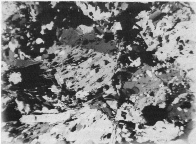
Plate 5. Twinned albite porphyroblasts with sieve structure and ragged outline in albite-quartz-muscovite schist from near North Duxbury (Loc. 16, Fig. 2), 30X, crossed nicols. The twinning is exceptional as most albite porphyroblasts show no twinning.
