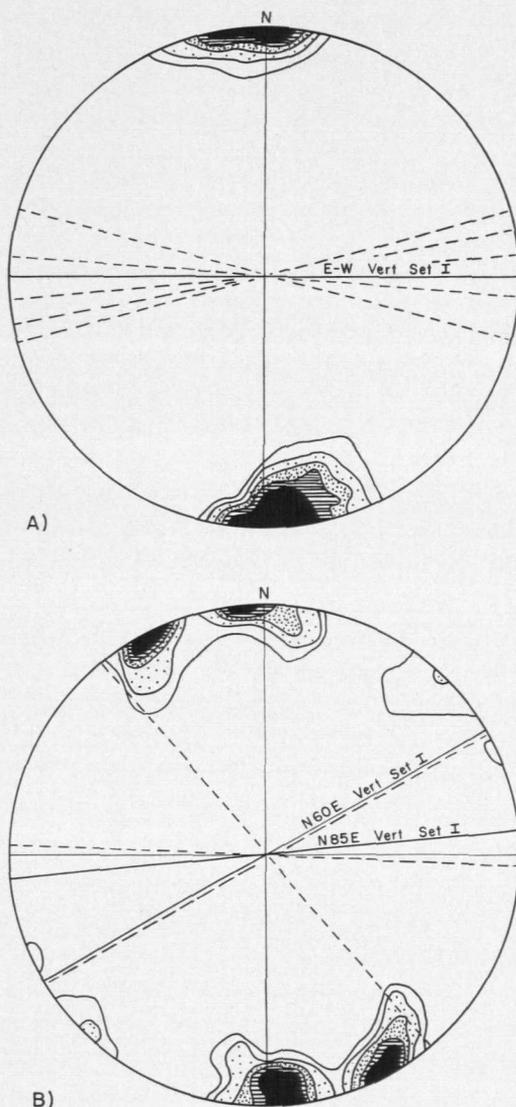
Figure 5. Joint diagrams for (A) east of Huntington (Loc. 36, Fig. 2) and (B) near Jonesville (Loc. 37, Fig. 2). Poles to 63 (A) and 97 (B) joints are plotted by projection on a lower hemisphere and contoured at 15-12-9-6-3 %. Bedrock is mica schist with attitude of (A) N.5°W. 60°SW. and (B) N.10°E. 85°SE. Broken lines are strike directions of lineations observed on aerial photographs at these respective localities.
