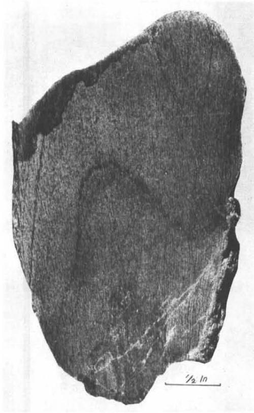
Figure 46. Photograph of a shadowy relict of an earlier ( $S_1$ ) fold cut by an extremely well-developed schistosity ( $S_1$ ), which is axial plane to the folds. Note the rippling of the schistosity at the bottom. From Barnes Brook, northeast of East Lyndon (G2816).
