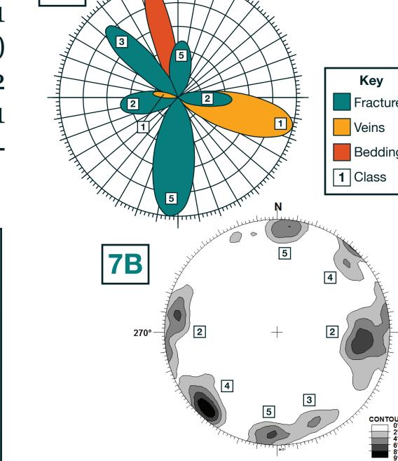
A) Rose plot of fractures, veins, and bedding. B) EAN for fractures.
