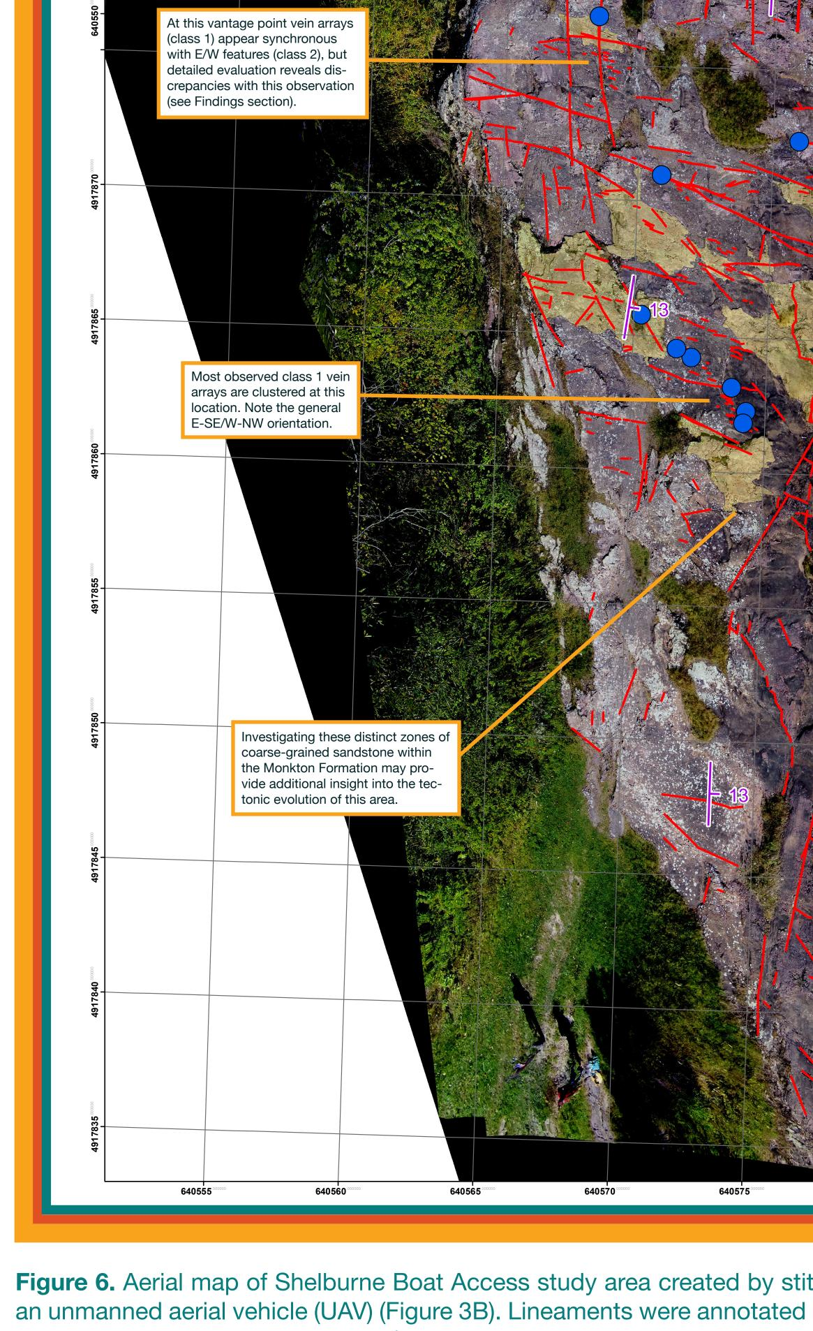
Figure 6. Aerial map of Shelburne Boat Access study area created by stitching together numerous aerial photos captured by an unmanned aerial vehicle (UAV) (Figure 3B). Lineaments were annotated (red lines) manually in GIS both before and after field data (blue dots and purple bedding measurements) was collected.
