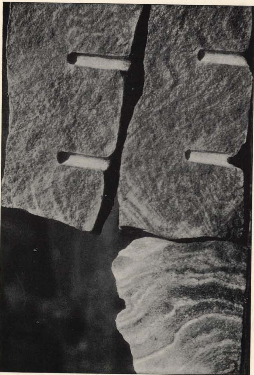
Blocks of Washington Limestone, Showing Banding as Seen on Freshly Broken Surfaces.
