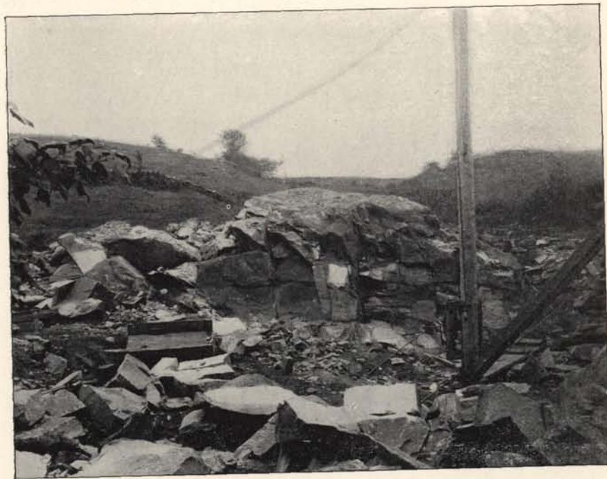
Quarry of Washington Limestone, Washington, Vt. Strike of rock N. 10^{\circ} E. Dip 15^{\circ} W.
