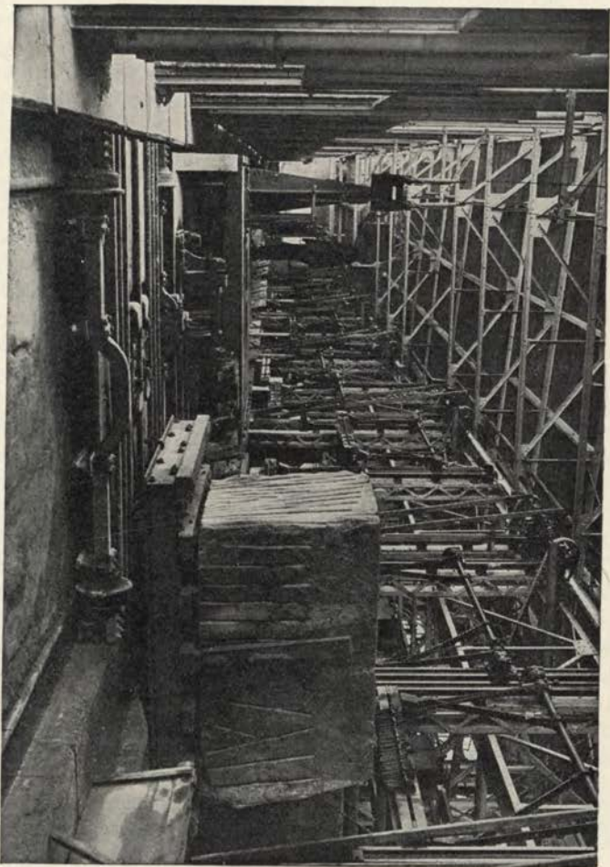
FIG. 44. Interior of a marble mill showing steel framework and electric transfer track for loading and unloading marble into gang saws at right.
