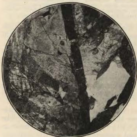
Photomicrograph of contact limestone at Crazy Creek. Magnification 30 diameters. Crossed nicols. The microphotograph shows actinolite characterized by the cross cleavage at 126° or by long needles, quartz (clear white) and carbonates (turbid).
