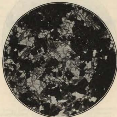
Photomicrograph of rock from the contact between the Bruce limestone and a quartz diabase sheet. Ordinary light. Magnification about 30 diameters. The photomicrograph shows garnet and diopside (light) and hornblende (dark) being replaced by magnetite (black).
