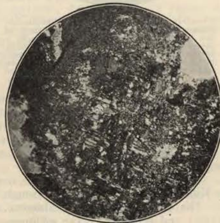
Photomicrograph of quartzite inclusion in granite showing small elongate areas of feldspar in the sericite aggregate. The feldspars are all approximately parallel as indicated by the cleavage and twinning planes. Crossed nicols. Magnification about 30 diameters.
