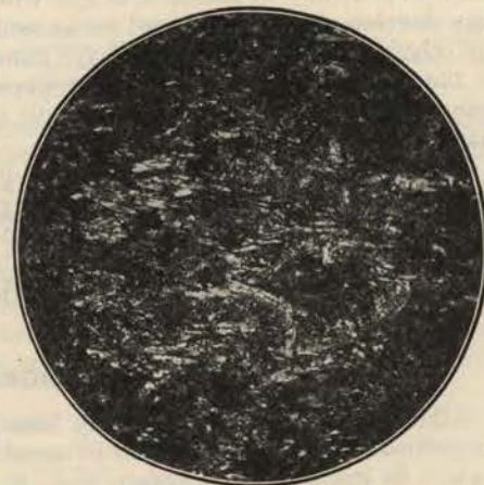
Photomicrograph showing rhombohedral shear lines in diabase porphyrite or Huronite. Magnification about 30 diameters. Ordinary light.
