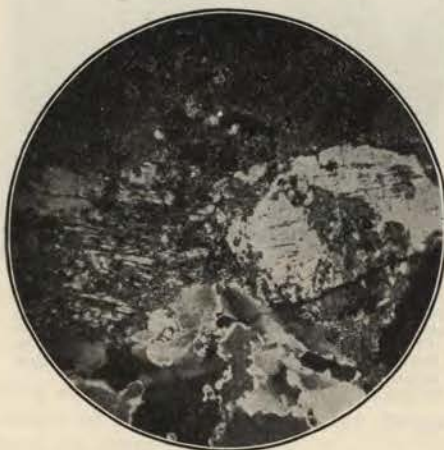
Photomicrograph of quartzite immediately adjacent to the granite showing many of the small feldspars joined up to make a larger one and surrounding lacunoid, turbid, areas of sericite. The rock closely resembles a granite in texture, structure, mineral and chemical composition. Crossed nicols. Magnification about 30 diameters.
