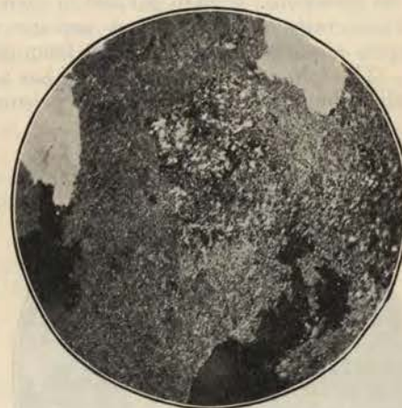
Photomicrograph showing sericitized Mississagi quartzite from the interior of a xenolith in the Killarney granite. The quartz (white) is almost completely altered to sericite. Crossed nicols. Magnification about 30 diameters.
