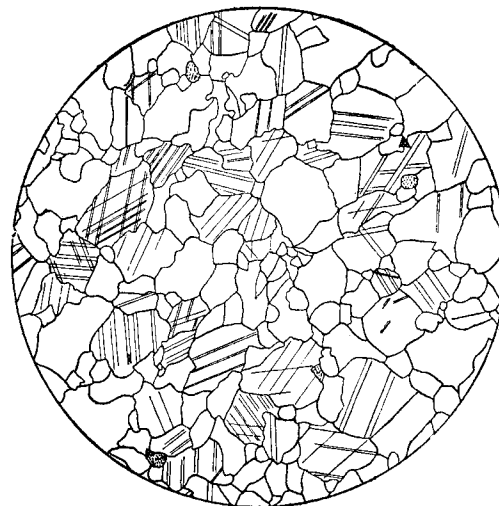
FIGURE 13.—Thin section of "white" calcite marble, "Dorset A," from the Norcross-West Valley quarry near South Dorset. Texture, grade 5. Dotted particles are quartz. Enlarged 20 diameters.
