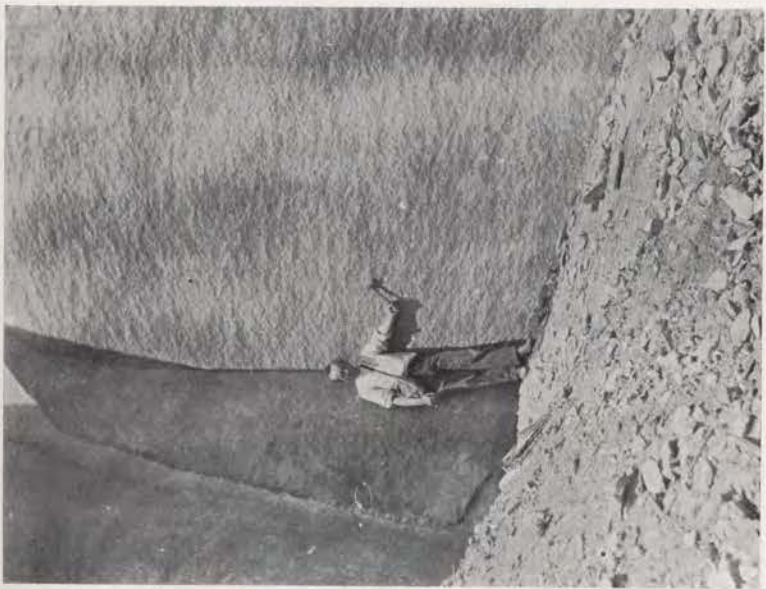
A. WOODBURY GRANITE CO.'S GRAY QUARRY, SHOWING THICKNESS OF A SINGLE SHEET, ROBESON MT., WOODBURY.
