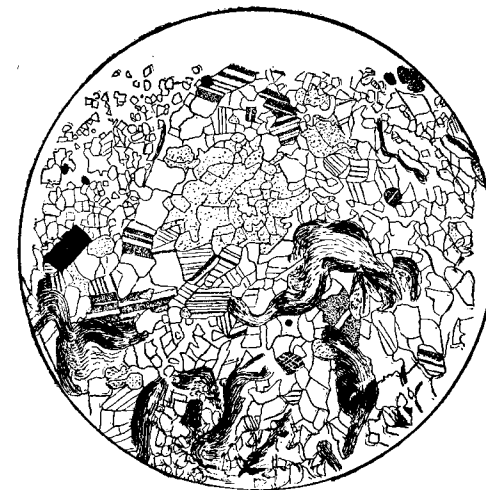
FIGURE 7.—Thin section of quartzose dolomitic and sericitic calcite marble from knoll near Brandon. Dotted particles are quartz; finer-grained area at upper left side is dolomite; the fibrous portions consist of sericite, which, where shaded, is graphitic; the black particles are pyrite; the larger clear particles and the banded particles are calcite. Enlarged 27 diameters.
