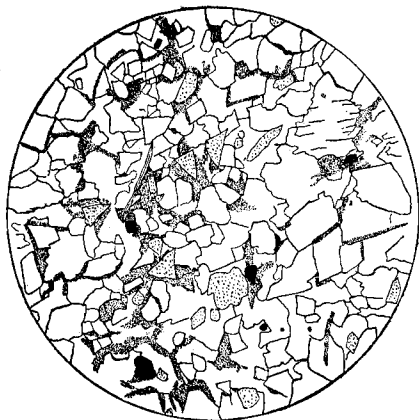
FIGURE 8.—Thin section of hematitic quartzose dolomite from Swanton. Dotted particles are quartz; black are magnetic; shaded areas are hematite stain; a black-banded particle is plagioclase, a long-streaked one, muscovite; the rest are dolomite. Enlarged 77 diameters.
