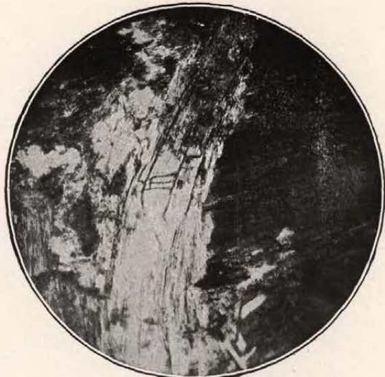
FIGURE 1.—PHOTOMICROGRAPH OF SECTION 89 Showing the cross-fibre and bifurcation of the amphibolite veins. The relation of the parts is such as to strongly suggest fracturing by shear-pressure.
