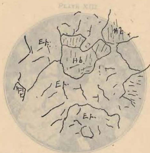
FIGURE 1.—SECTION (10) OF THIN-SECTION (1) CONTAINING LARGE QUANTITIES OF EPIDOTE AND HORNBLENDE. SECTION BEING EXAMINED UNDER A MOUNT OF POLARIZED LIGHT.
