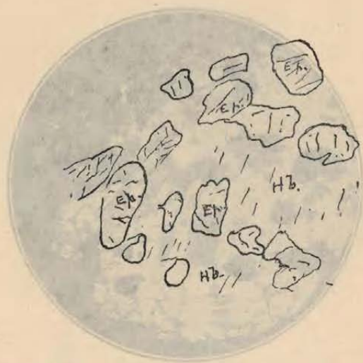
FIGURE 2.—SECTION (11) CONTAINING LARGE QUANTITIES OF EPIDOTE AND HORNBLENDE. SECTION BEING EXAMINED IN CIRCULAR POLARIZATION. PHOTOGRAPH TAKEN BY DR. J. W. HAYES.
