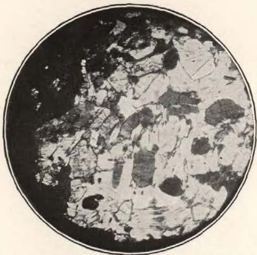
FIGURE 2.—AMPHIBOLITE (SECTION 45) CONTAINING LARGE AMOUNT OF GRANULATED EPIDOTE EMBEDDED IN CRUSHED HORNBLLENDE. PHOTOMICROGRAPHS OF AMPHIBOLITE.
