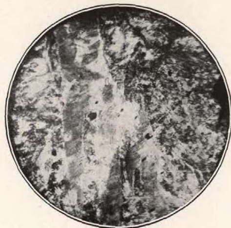
FIGURE 2.—SECTION (4) A OF TYPICAL COARSE AMPHIBOLITE Showing the curved cleavage partings in a large hornblende. PHOTOMICROGRAPHS OF AMPHIBOLITE.
