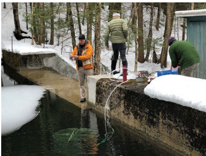
Figure 2. Sampling surface water in Bennington for tritium, isotopes and water chemistry. Age dates are a component of the aquifer characterization project in Bennington.
