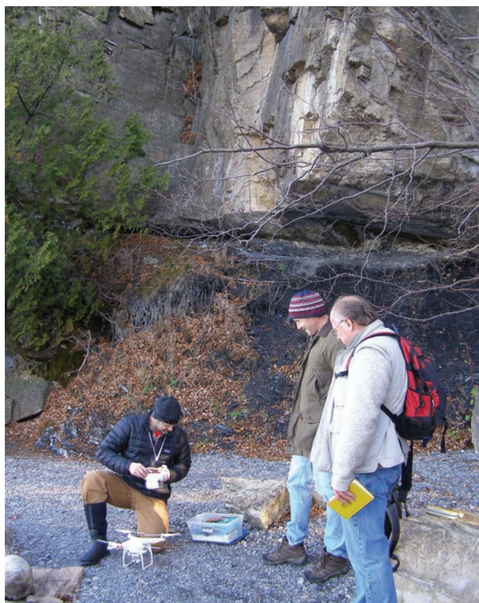
Figure 1. Setting up for a drone flight at the Champlain Thrust in northwest Vermont. The drone is useful for mapping and interpreting fractured bedrock at specific sites.
