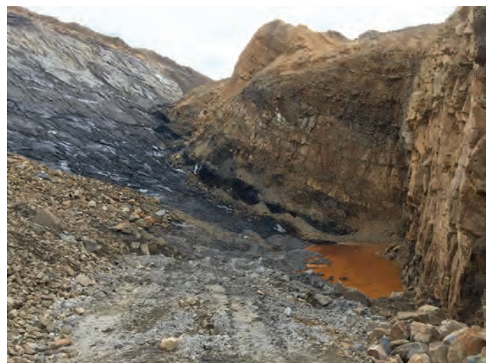
Figure 1. Strip mine in western Broad Top coalfield on Kelly coal (7 ft thick) along limb of third-order, northeast-trending syncline. Beds in photo dip about 40°NW.
