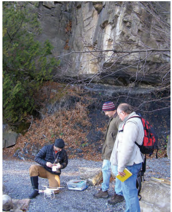
Figure 1. Setting up for a drone flight at the Champlain Thrust in northwest Vermont. The drone is useful for mapping and interpreting fractured bedrock at specific sites.
