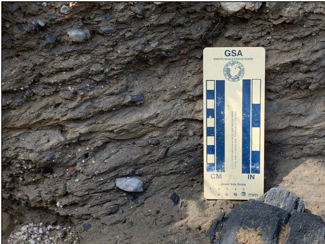
Figure 5: Glacial till exposed in erosional gully between Newport and Derby. Fissility in the till may result from shear stresses applied during movement of the overlying ice sheet.
